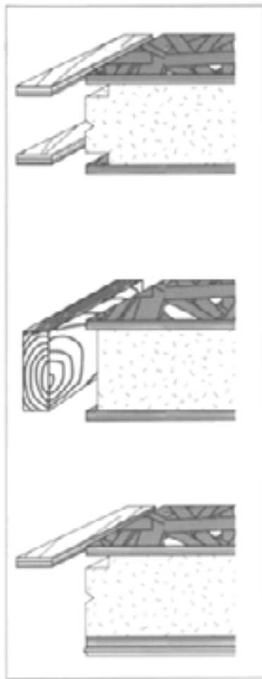
Figure 1. There are three common methods of joining panels: a dual plywood spline joint (top), a solid 2x blocking
